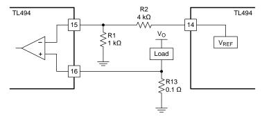
Figure 12. Current-Limiting Circuit
