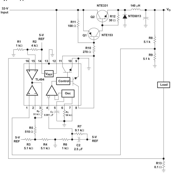
Figure 9. Switching and Control Sections
