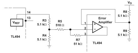
Figure 11. Error-Amplifier Section
