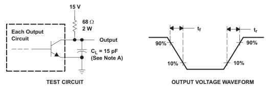
NOTE A:  $C_L$  includes probe and jig capacitance.
