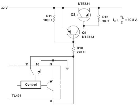
Figure 15. Power-Switch Section
