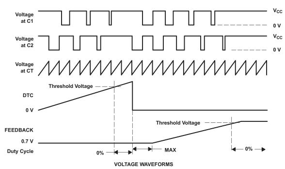
Figure 5. Operational Test Circuit and Waveforms
